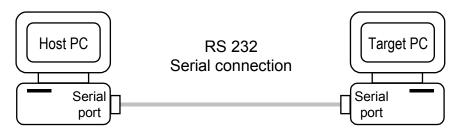
For detailed information on setting up the hardware and software for serial communication, see "Serial Communication" on page 2-11.
