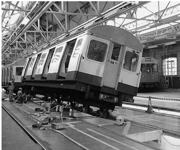
FIGURE 13.32 Sway test. Source: Photo — courtesy of Serco Railtest Ltd.
