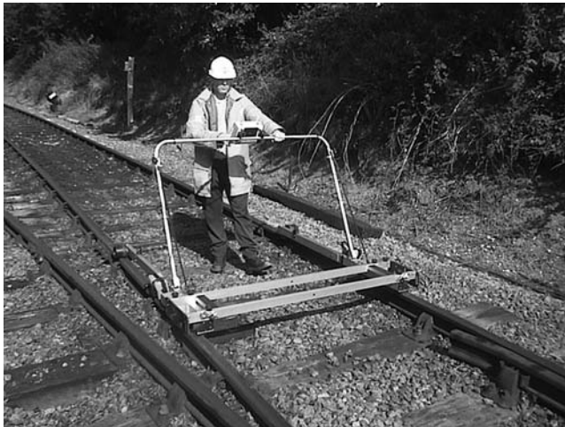
FIGURE 13.25 Track geometry recording trolley (courtesy of Abtus Ltd.). Source: Abtus Ltd. — Catalogue. With permission.
