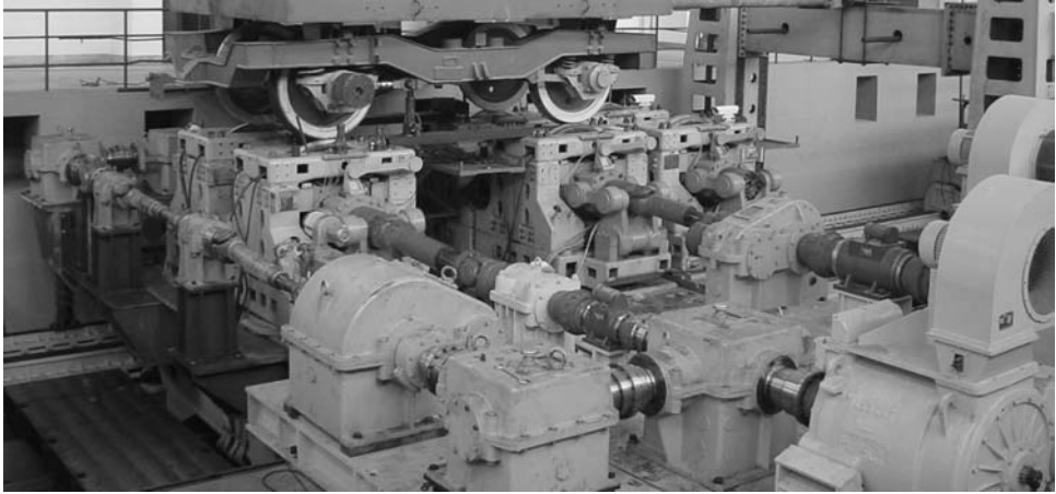
FIGURE 14.10 The roller rig with differential driving system.
