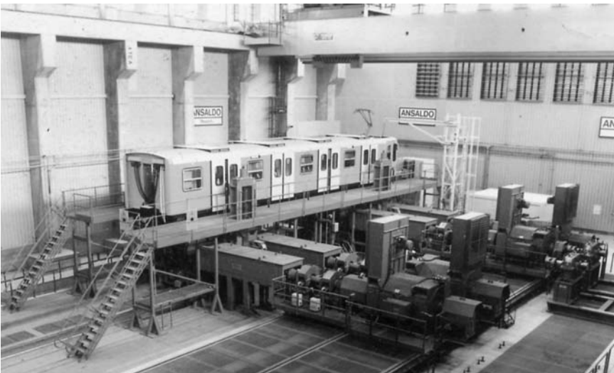
FIGURE 14.11 Overview of the Naples roller rig.
