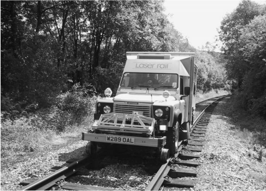
FIGURE 7.5 Road–Rail laser gauging vehicle, operated by Laser Rail Ltd.
